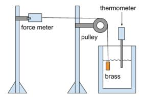
I repeated my experiment with the addition of a pulley, set up like the figure above. Attaching the force meter to a clamp stand also removed errors caused by my hand moving while holding it.
