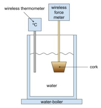
The experiment was set up as shown in the figure above.
