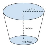
The piece of cork used for my experiment had the shape of a truncated cone with the measurements as shown on this figure.
